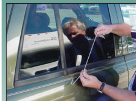
4. Wedge open the weather-stripping on the rear door as far to the rear as possible.
